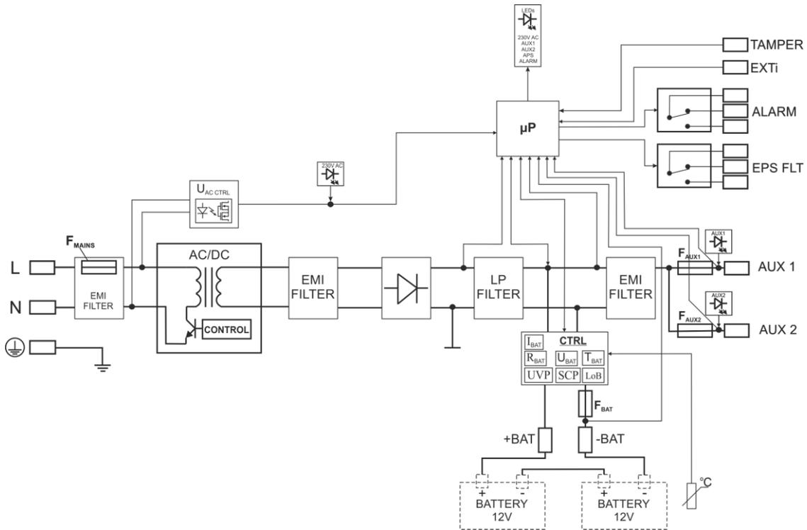
Fig. 1. PSU block diagram.
